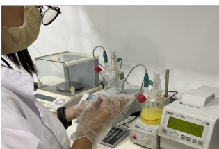
Transformer Oil Testing
